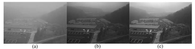
Fig 1. Intensity component of (a) hazy image, (b) dehazing with MDCP, (c) luminance enhancement with our propose.
