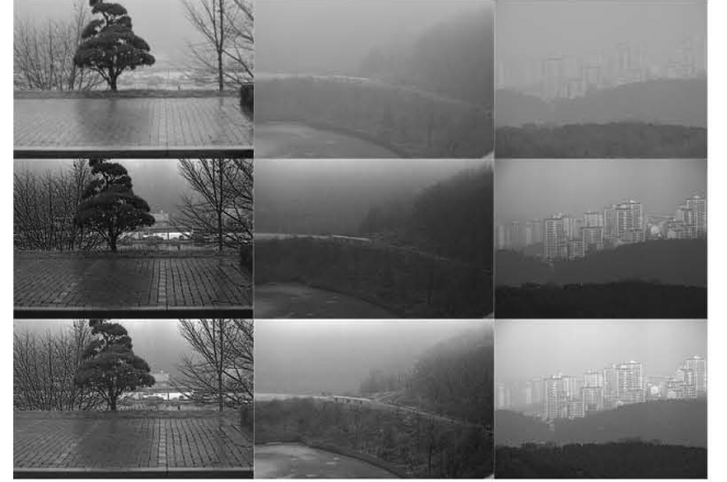
Fig 3. Compare our propose and MDPCP (a) first row: dense-haze image, (b) second row: MDPCP, (c) third row: our propose
