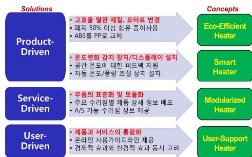
Fig. 2 Eco-design method for electrical small heater
