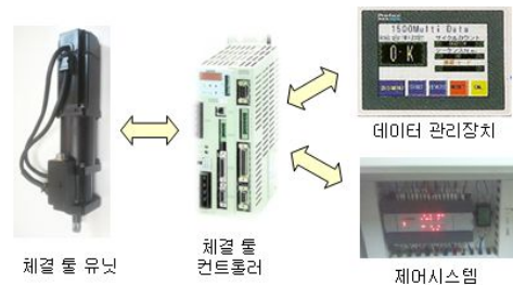
Fig. 1 Conceptual diagram of automatic tightening system
