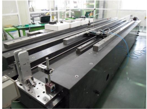
Fig. 4 Measurement of rail profile
