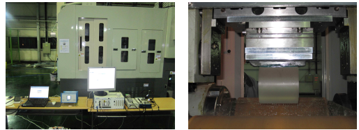
Fig. 1 Experiment setup for diamond wire saw cutting of sapphire ingot
