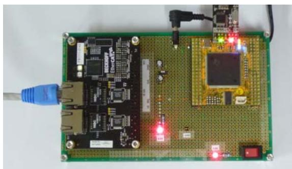
Fig. 3 DSP based EtherCAT Slave
