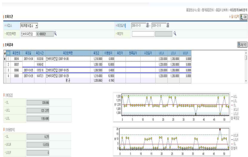
Fig. 2. The I-MR Control Chart Results for the 180kVA IGBT-SIV
