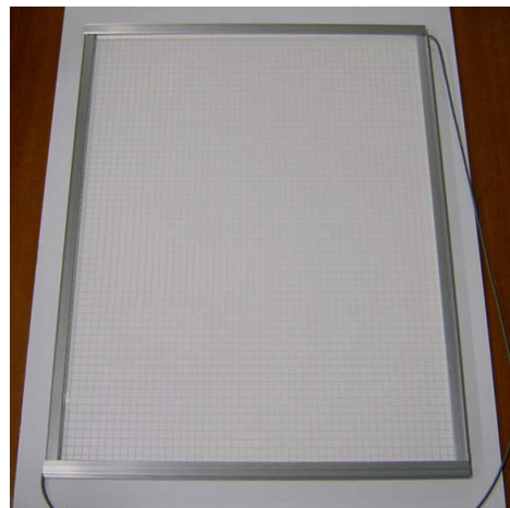
Fig. 1 Photograph of the fabricated light guiding plate as an illumination system for photobioreactor
