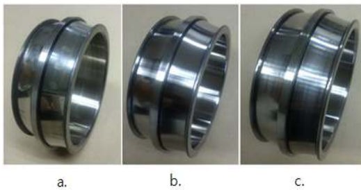
Fig. 2 Remanufacturing process (a. untreated, b. polished, c. UNSM treated)
