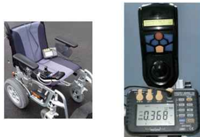
Fig. 4 Prototype powered wheelchair and result of energy consumption test
