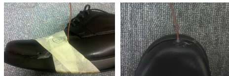
Fig. 1 Sensor location on toe and midsole
