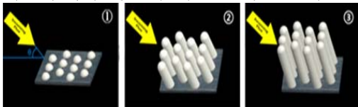
Fig. 1 Schematics of the process of fabricating the nanorod structure
