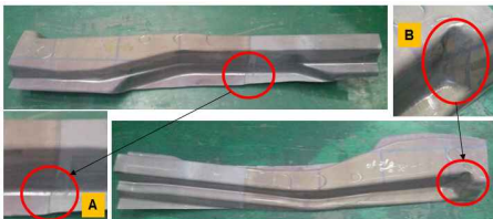
Fig. 3 Appearance of part after press hardening
