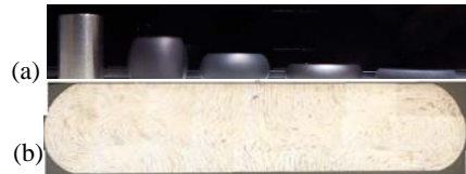
Fig. 1 Configuration of a specimen deformed by compression and internal material flow, (a) The change of the specimen by compression rate 0, 30, 50, 70, 90%, (b) the section that is cut in the compression direction of a 70% compressed specimen
