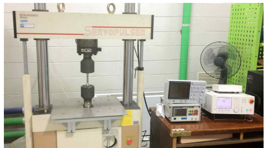
Fig. 1 Fatigue testing machine and Ultrasonic test instrument
