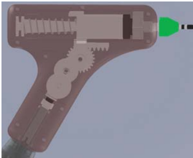
Fig. 2 Driving mechanism of membrane sinus lift system
