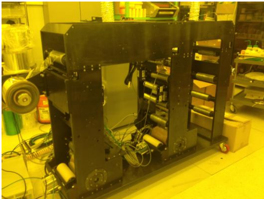
Fig. 2 Manufactured experimental platform for web handling research
