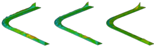
Fig. 4 Subsequent deformed shapes of the panel during the roller hemming process with CAE
