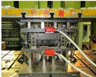
Fig.3 Die for warm deep drawing
