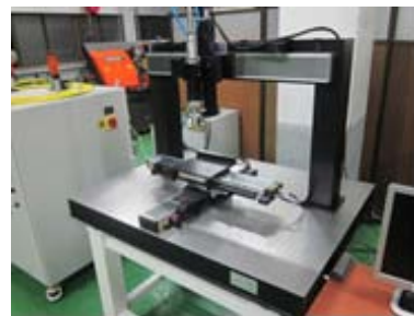
Fig. 2 Photograph of laser forming test-bed
