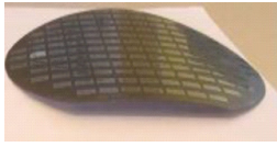
Figure 2. Warpage evolution of typical EWLP wafer.
