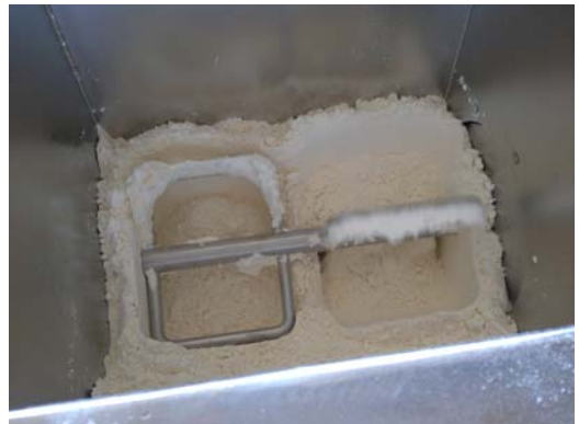
Fig. 2 Clogging effect of flour caused by rotating agitator
