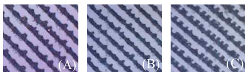
Fig. 3 The effect of doctor tip shape on printability: thickness of 0.15 mm, pressure of 5 bar and velocity of 5 m/min applied. (A) bevel, (B) lamella, (C) round
