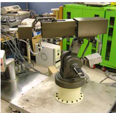
Fig. 1 Configuration of RS2(6-axis articulated robot)
