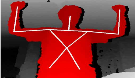
Fig 2 Joint data using OpenNI / NITE library
