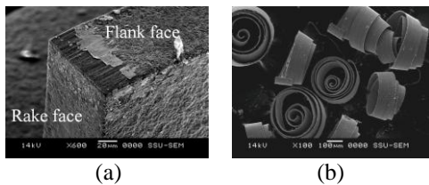
Fig. 3 SEM of (a) PCBN tool after machining and (b) cutting chip
