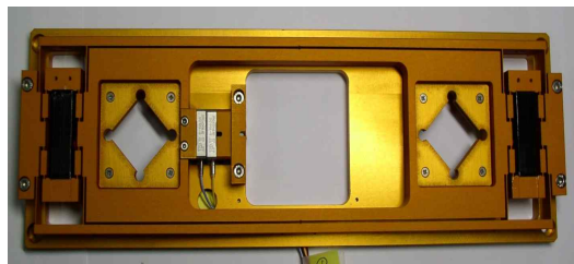
Fig. 1 Piezo stage driven by antagonistic piezo forces
