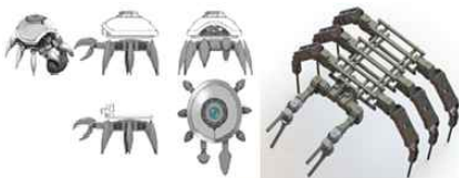
Fig. 1 Composition of Animatronics Robot
