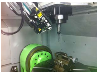
Fig 6. Experimental set-up for laser-assisted machining
