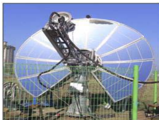
Fig 2. Solar Dish System (INHA-DISH)
