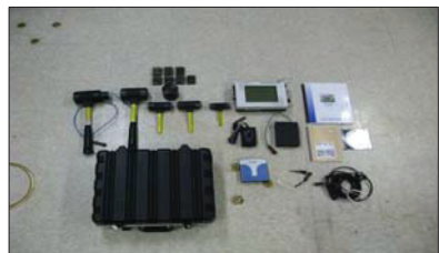
Figure 3 Pile Integrity Tester Set
