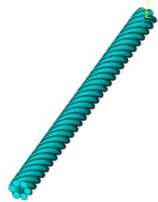
Fig. 1 Overall shape of guidewire.
