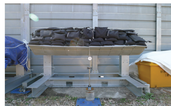
(a) post interval: 2 m (test load: 3.6 kPa)
