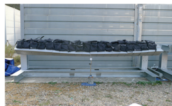
(b) post interval: 4 m (test load: 1.6 kPa)
