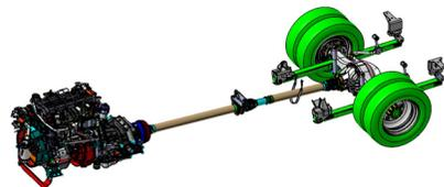
Fig. 3 County Bus Driveline Layout
