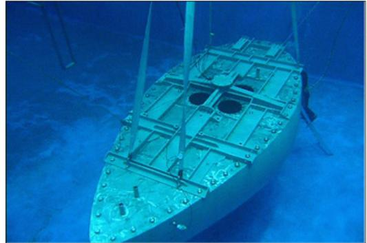
Fig. 1 Modal test of FRP structure in water
