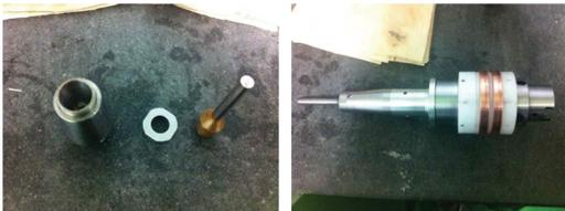
Fig. 3 Made of detachable ultrasonic tool horn
