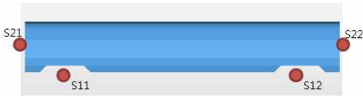
Figure 2 Noise source of High Speed Train at the Bogie and Inter-Coach Space
