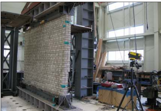
Figure 3. Measuring of vibration characteristics
