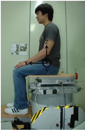
Fig. 2 vibration exciter and subject sitting on the rigid seat
