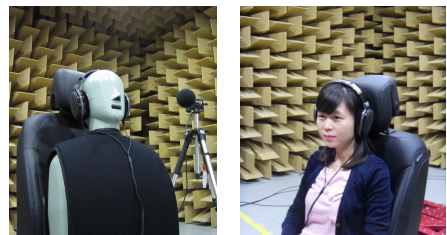
Fig. 4 Photography of objective evaluation with the head & torso simulation system and human's subjective evaluation
