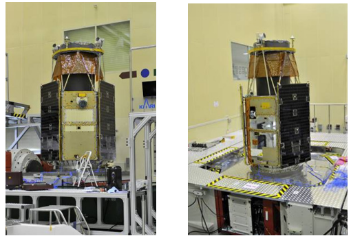
(a) lateral direction (b) axial direction Fig. 1 Sinusoidal vibration test configuration
