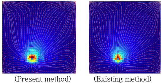
Fig. 1 Vibration intensity (1m x 1m plate)
