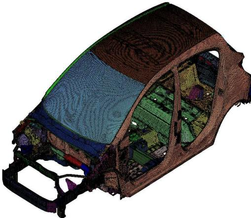
Fig. 1 Finite elements model of body structure
