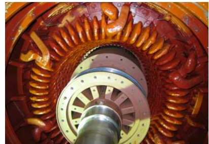
Fig.1 Photograph of 100MW class electrical generator
