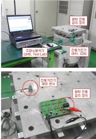
Fig. 3 Test setup
