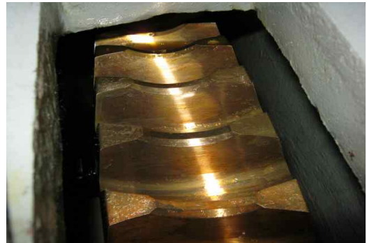
(b) No pitting on gear tooth of up direction
