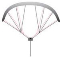
Fig.3 Actuator located between the bridle points
