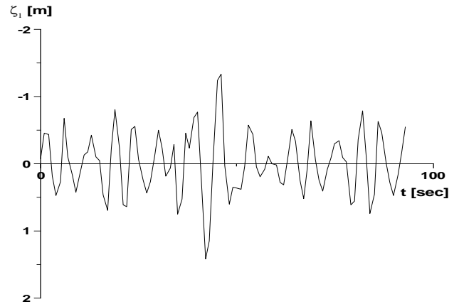
Fig. 1 Estimated time history of wave elevation at fixed position of seas ; Beaufort scale 5
