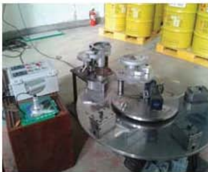
Fig.2. The dismantling equipment of RSR.
