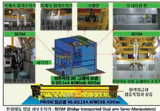
Fig. 3. Schematics of a developed RHEM (Remote Handling Evaluation Mock-up).
